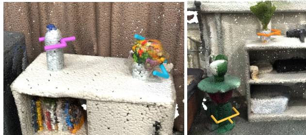
Figure 4. Grasping Result. Visualization of computed grasp poses for a milk bottle , some flowers , a side table , and a plant .
