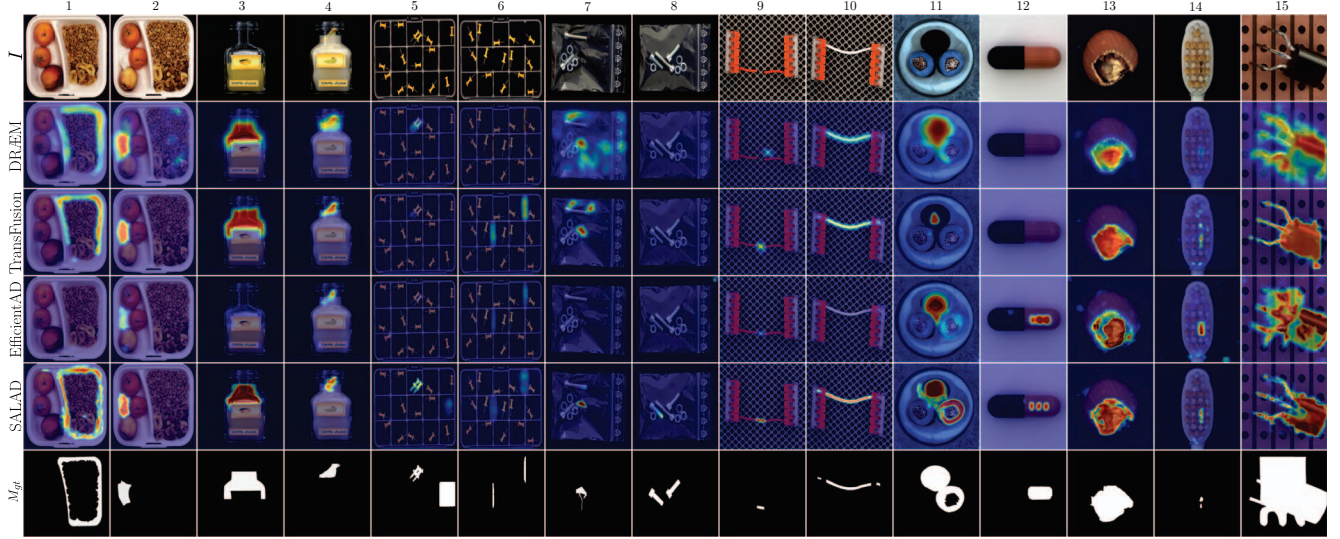
Figure 5. Qualitative comparison of the anomaly segmentation masks produced by SALAD and three other state-of-the-art methods. In the first row, the image is shown. In the next four rows, the anomaly segmentations produced by DRÆM [42], TransFusion [12], EfficientAD [1] and SALAD are depicted, and in the last row, the ground truth mask is depicted. For SALAD, we visualized the sum of A_a and A_c (the outputs of the appearance and the composition branch).
