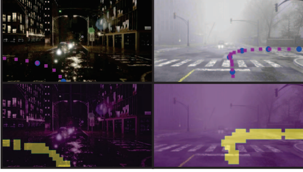
Figure 4. Action Mask. In the top row, we show two examples of the RGB image with the path (purple) and waypoints (blue) projected onto it. Patches containing a path or waypoint are marked as 1 (yellow), and all other patches are marked as 0 (purple), creating the binary mask, overlaid on the image below for visualization.
