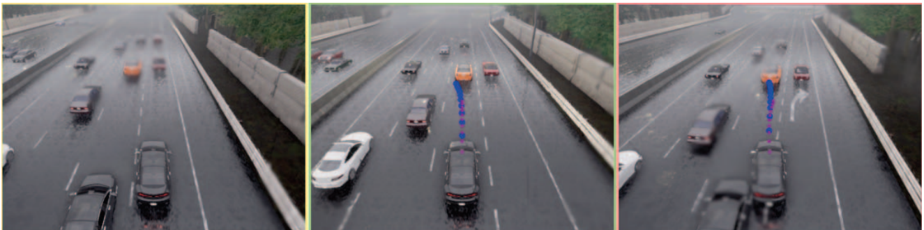
Figure 6. Lane Change without Forecasting. Left: The initial state of the scene, where the ego vehicle is tasked with switching to the left lane. Middle: The Async Model successfully executes the lane change while avoiding collisions by leveraging forecasting. Right: The version without forecasting ( A ) fails to anticipate the future position of the vehicle behind, resulting in a rear-end collision. The predicted action for each model is overlaid on the image, with waypoints shown in blue and the path in red.
