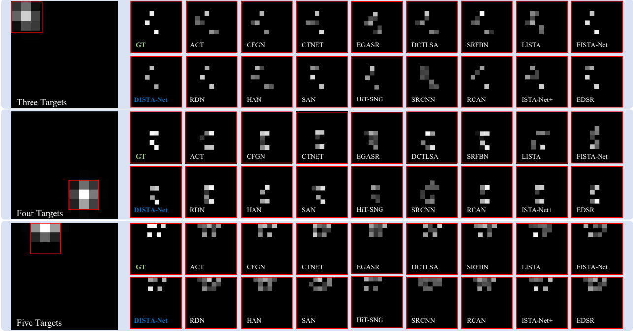
Figure 5. Visual comparison of 3\times sub-pixel division reconstruction for scenes containing different numbers of closely-spaced infrared small targets. The red boxes highlight regions where targets exhibit significant sub-pixel characteristics.
