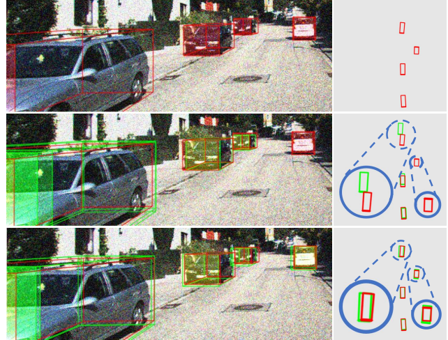
Figure 6. Qualitative examples on KITTI-C. In each row, we provide the front view (left) and the bird’s-eye view (right) visualizations. Red represents the ground truth of boxes, while Green represents the predictions. We circle some objects to highlight differences in predictions. The first row corresponds to the source model, the second to MonoTTA, and the third to our method.
