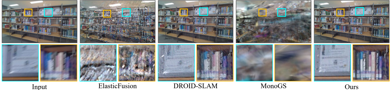
Figure 1. We propose a robust 3D scene reconstruction method from RGB-D input that effectively addresses extreme motion blur. Our approach achieves accurate camera poses and dense point clouds, producing clearer, deblurred scenes compared to existing methods.
