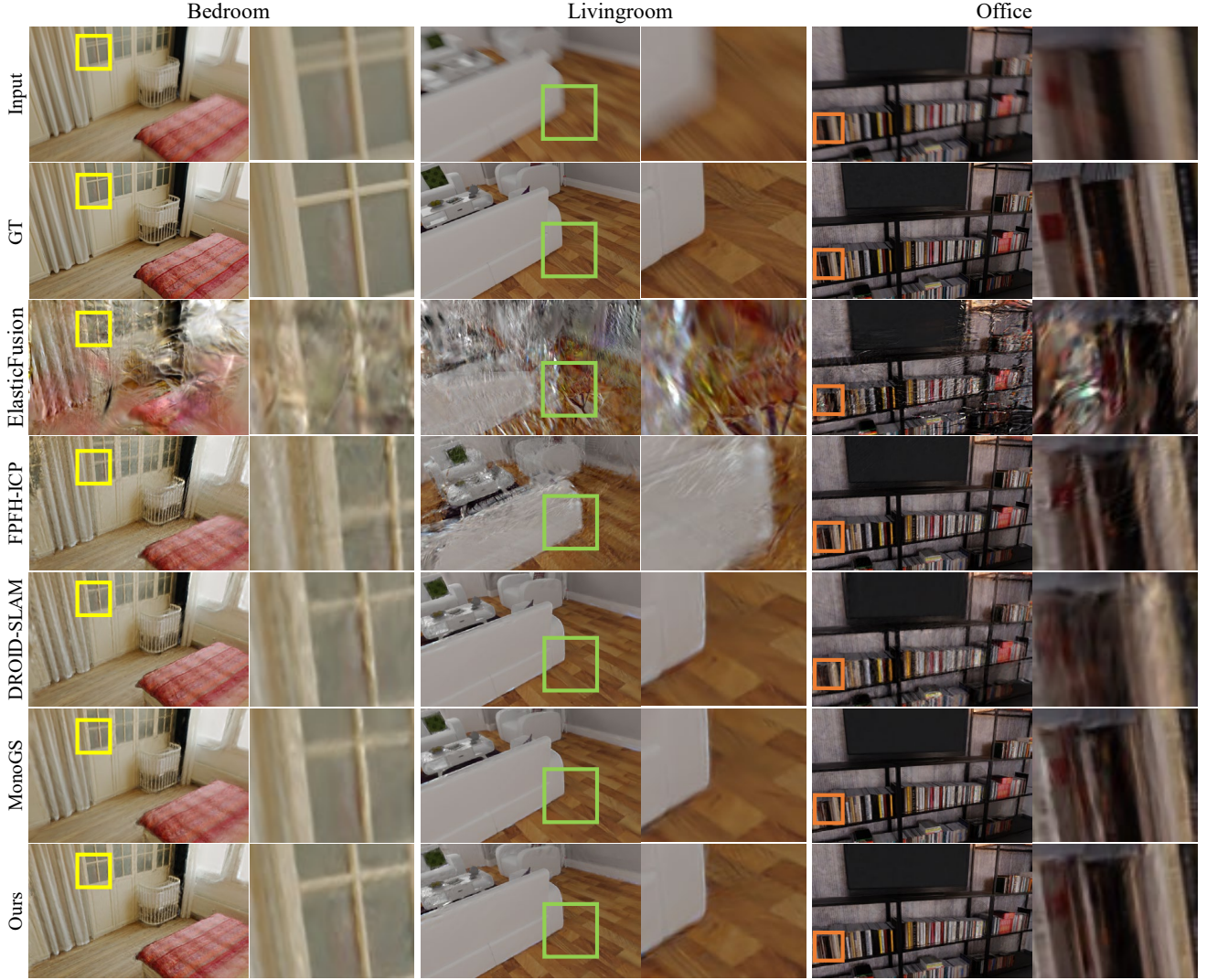
Figure 6. Qualitative comparison of deblurring performance from a novel view. Our method excels in restoring high-frequency details, whereas several methods, including COLMAP [31], fail under severe motion blur conditions (see Section 4.1). The corresponding quantitative results are provided in Table 2.
