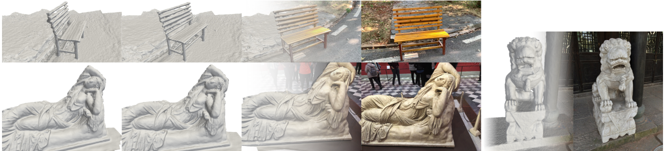
Figure 1. Examples of reconstruction meshes obtained within 3 minutes from sparse pose-free images via our method. We used here 6 (left) and 3 (right) input images respectively from scenes of datasets MVImgNet [97] and BlendedMVS [92].
