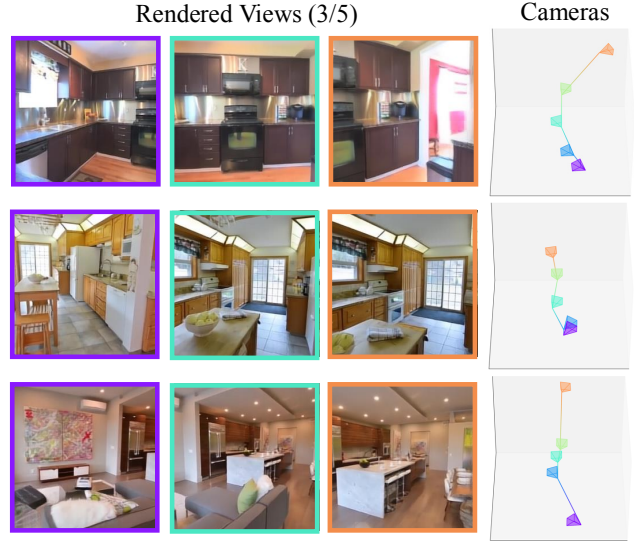
Figure 6. Visualization of RayZer predicted cameras learned with self-supervision. We visualize 3 out of 5 rendered views due to space limit, where the image index is highlighted by its color.
