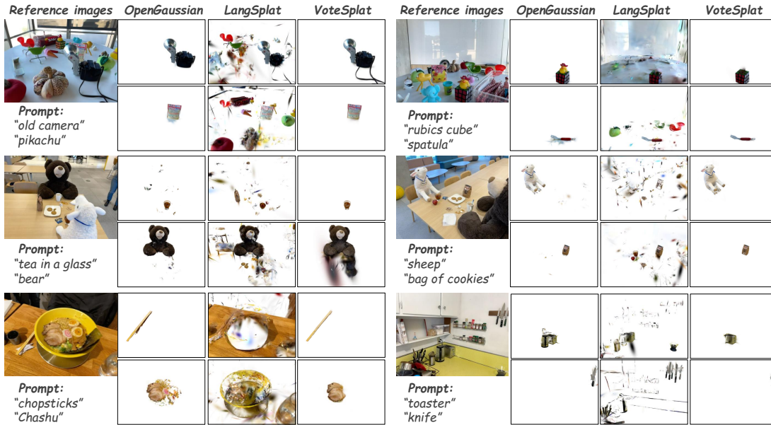
Figure 5. Open-vocabulary 3D object selection on the LERF dataset. VoteSplat outperforms LangSplat and OpenGaussian in accurately identifying 3D objects corresponding to text queries.
