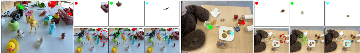
Figure 4. Click-based 3D object selection and scene editing results. VoteSplat enables complete 3D object selection without issues of incompleteness or redundancy. Moreover, after removing the selected Gaussian primitives, the scene can be effectively edited.
