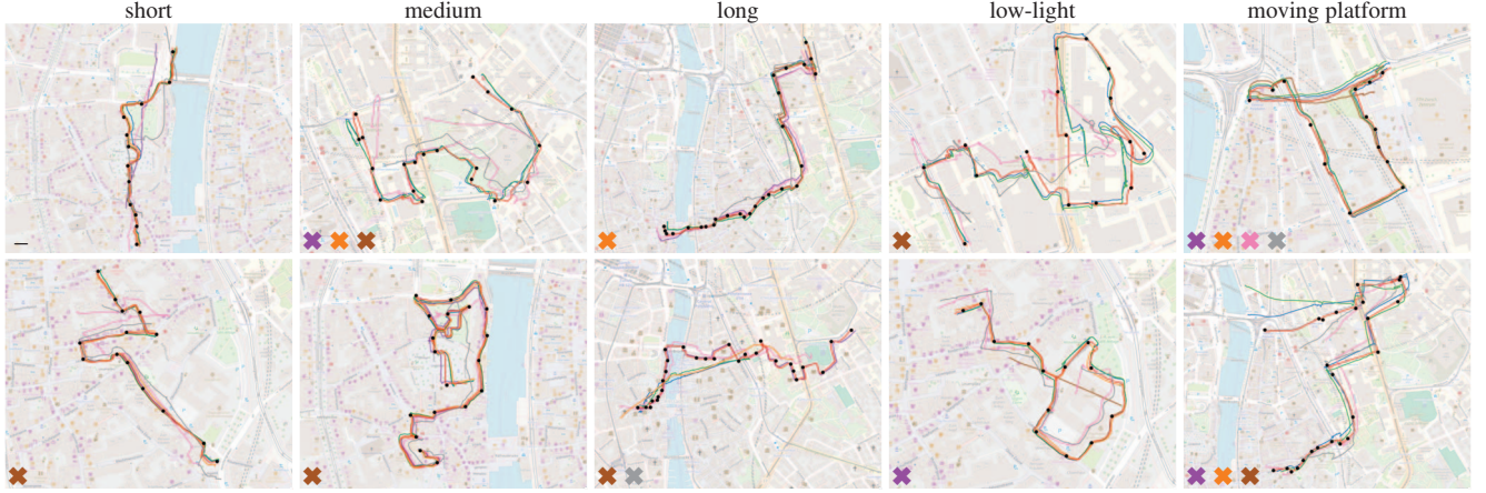
Figure 8. Visualizations of the trajectories estimated by different systems: OpenVINS ●, OpenVINS+Maplab ●, ORB-SLAM3 ●, OKVIS2 ●, Kimera VIO ●, DPVO ●, DPV-SLAM ●, and Aria’s SLAM ●. Failures are shown as ✕ and control points in black ●.
