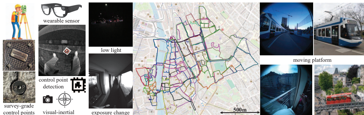
Figure 1. We introduce a dataset to benchmark multi-sensor VIO/SLAM with egocentric data at city scale. We record hours and kilometers of trajectories with Project Aria devices [21], with pose annotations derived from centimeter-accurate surveyed control points. We cover unique challenges of egocentric data, including low light, exposure changes, moving platforms, time-varying calibration, etc.
