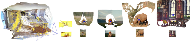
Figure 3. Scene scale mismatch. Point clouds reconstructed from metric depth estimation (RGB) are robust and unified, whereas SfM reconstructions (yellow) are relative-scale that may vary across frames. Our alignment enables relative-to-metric conversion of scene scale for real-world applications.
