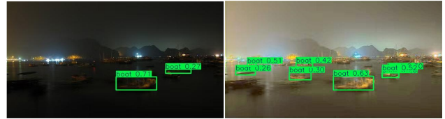
Figure 7. A visual comparison of the object detection task in low-light scenes (left) and scenes enhanced by GM-MoE (right).
