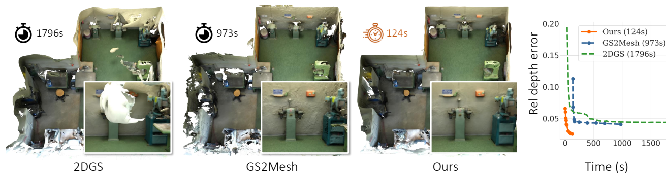
Figure 1. QuickSplat performs surface reconstruction of large indoor scenes from multi-view images as input. We learn strong priors for initialization of gaussian splatting optimization for surface reconstruction, as well as for per-iteration joint densification and gaussian updates. This results in high-quality mesh geometry that more accurately models flat wall structures as well as object details, while optimizing significantly faster than baselines.
