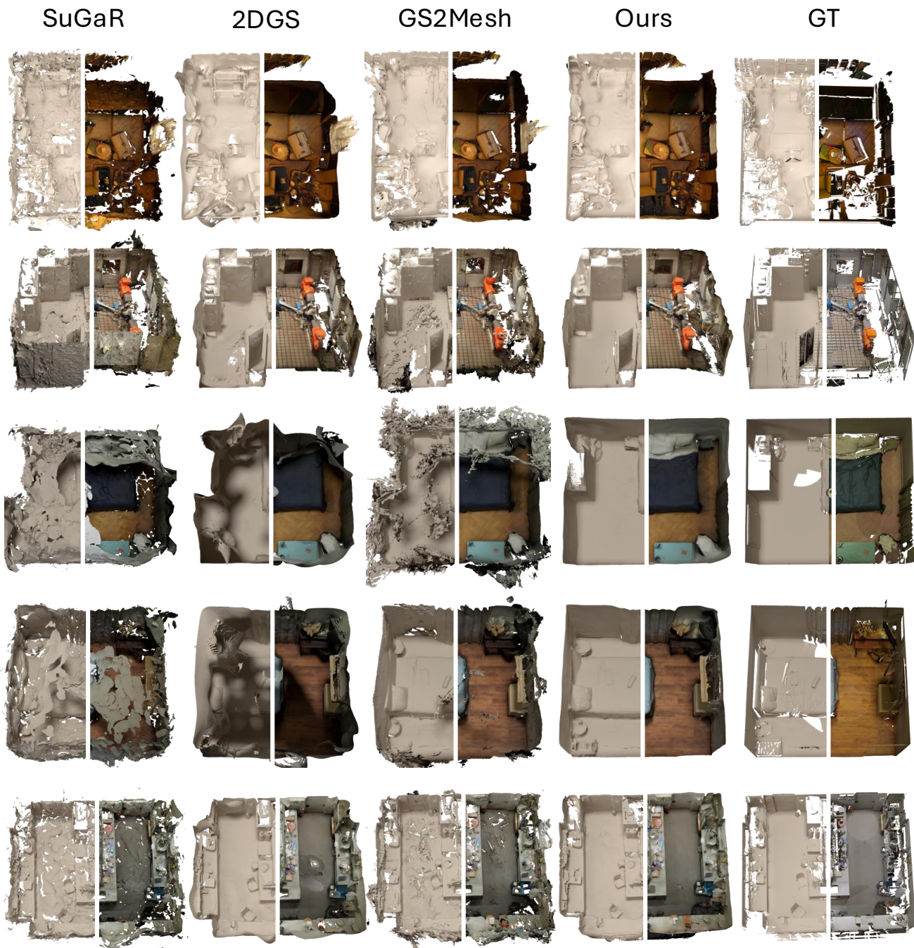
Figure 4. Qualitative comparison against baselines. We show top-down views of reconstructed mesh geometries (with and without vertex colors) in comparison to the ground-truth meshes of ScanNet++ [52]. Our method more accurately models flat wall structures and objects details, while producing fewer floating geometry artifacts.
