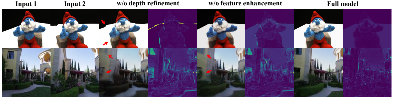
Figure 7. Ablation of fusion strategy. The 1st row is from small-baseline dataset DTU, and the 2nd row is from large-baseline dataset RealEstate10K. Our proposed fusion strategy works well with the area with occlusion or out of overlap.
