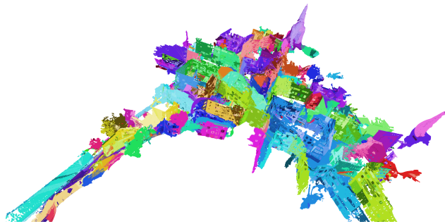
Figure 1. Point Cloud of Scene LIN from the LaMAR dataset [23]. Large object instances (e.g., houses) are distinctly colored, with their components (e.g., windows) shaded in a darker variant of the same color to indicate hierarchical relationships.
