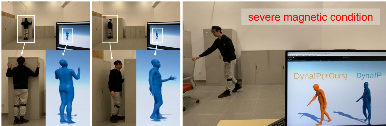
Figure 1. We propose MagShield, an IMU orientation estimation method that specifically designed to address magnetic disturbances in sparse inertial MoCap systems. By integrating with our method, existing sparse inertial MoCap systems (left, PNP; right, DynaIP) can operate reliably even under severe magnetic condition.
