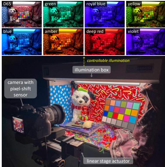
Figure 4. Dual-camera MS-RGB capturing system.
