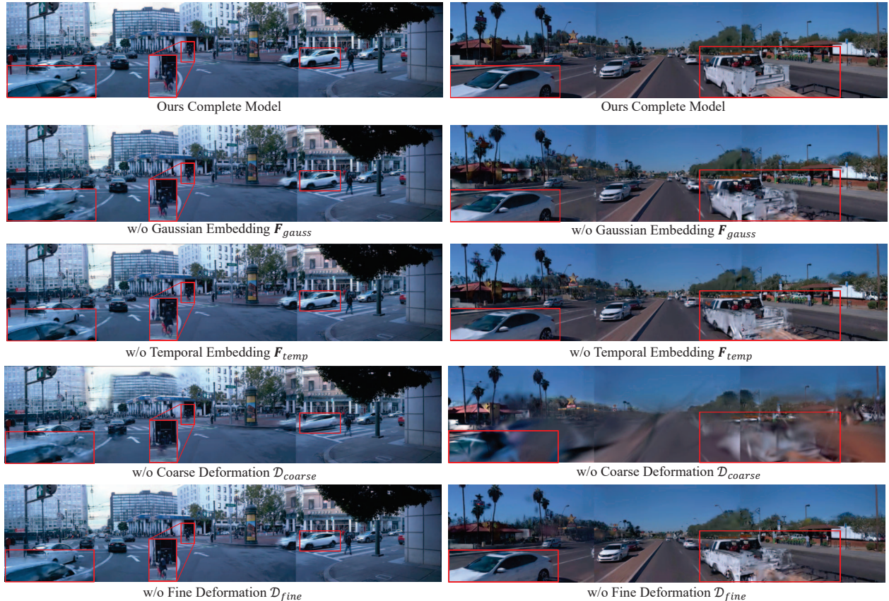
Figure 6. Qualitative ablation study results across three camera views from the Waymo dataset. (a) Our complete model achieves sharp and consistent reconstruction. (b) Removing Gaussian embedding \mathcal{F}_{gauss} leads to blurry object boundaries. (c) Without temporal embedding \mathcal{F}_{temp} , results show motion artifacts. (d) Without coarse deformation \mathcal{D}_{coarse} , geometric consistency is lost. (e) Absence of fine deformation \mathcal{D}_{fine} causes detail degradation.
