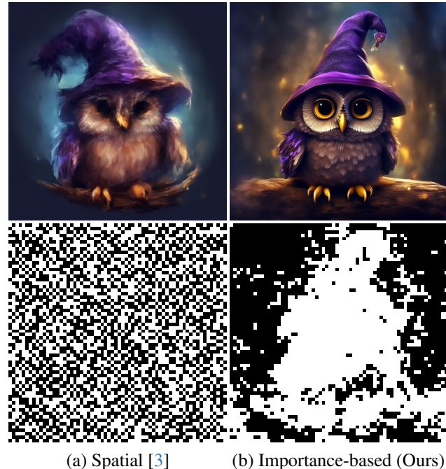
Figure 1. Importance-based Token Merging. Our method prioritizes important tokens during token merging, resulting in images with greater details in essential areas compared to ToMeSD [3]. In the second row, we show the regions (in white) where computation (e.g., attention) will take place after token merging.
