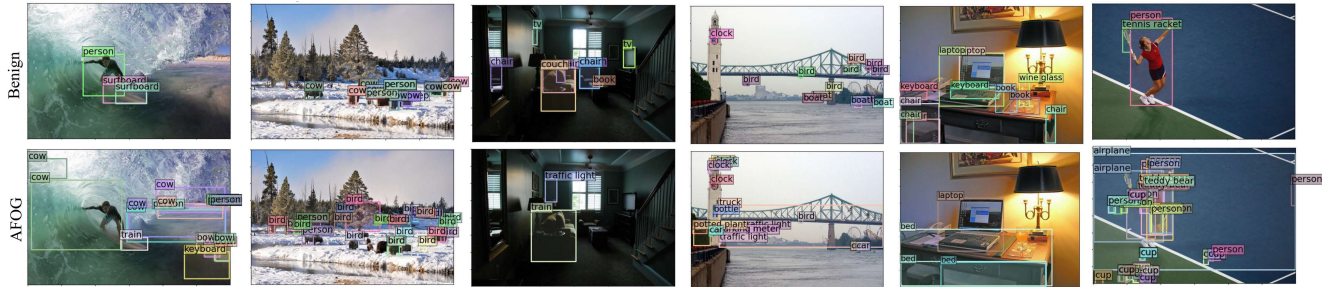
Figure 4. Visualization with six examples, comparing benign scenario and AFOG attack results on Detection Transformer (DETR) with ResNet-50 backbone. Six diverse test images contain objects with varying classes, scales, perspectives, lighting, motion, and textures.
