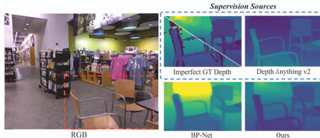
Figure 2. Existing depth completion methods, such as BP-Net [32], trained solely on noisy ground truth or simple colored depth, fail to recover high-frequency details. In contrast, depth foundation models like Depth Anything v2 [43] excel at generating detailed pseudo depths. We propose leveraging their high-frequency knowledge to enhance depth completion.
