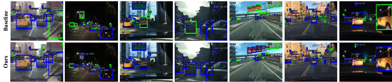
Figure 4. Detection results on ID dataset . Here we use Berkeley DeepDrive-100k dataset as ID dataset. We use RegNetX4.0 and Transformer as backbone. The first row is the detection results of baseline [6]. The second row is the detection result of our APLGOS. Our APLGOS rarely misclassifies the ID class as OOD class, and there is almost no missed detection.
