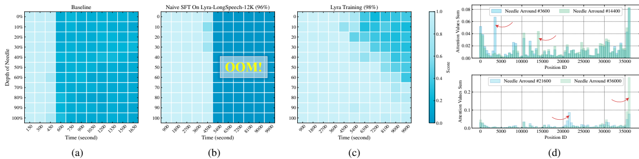
Figure 6. Comparison of needle in long speech haystack (average with five samples). (a) The baseline model can not retrieve right needles after 450 seconds. (b) Model finetuned on our long speech datasets can not retrieve right needles after 4,500 seconds and achieves 96% accuracy in 4,500 seconds. (c) Our latent extractor, trained on our long speech datasets, can retrieve longer audio (9,900 seconds), and presents 98% accuracy in 4,500 seconds. (d) As the position of the needle changes, the attention in our model also shifts accordingly.
