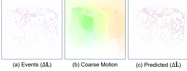
Figure 2. An example (corresponding to the jelly cube in Fig. 1(b)) of coarse motion through optimization. The predicted brightness change (c), denoted as \Delta\hat{\mathbf{L}} in Eq. (5) aligns well with the event frame (a), represented by \Delta\mathbf{L} in Eq. (4).
