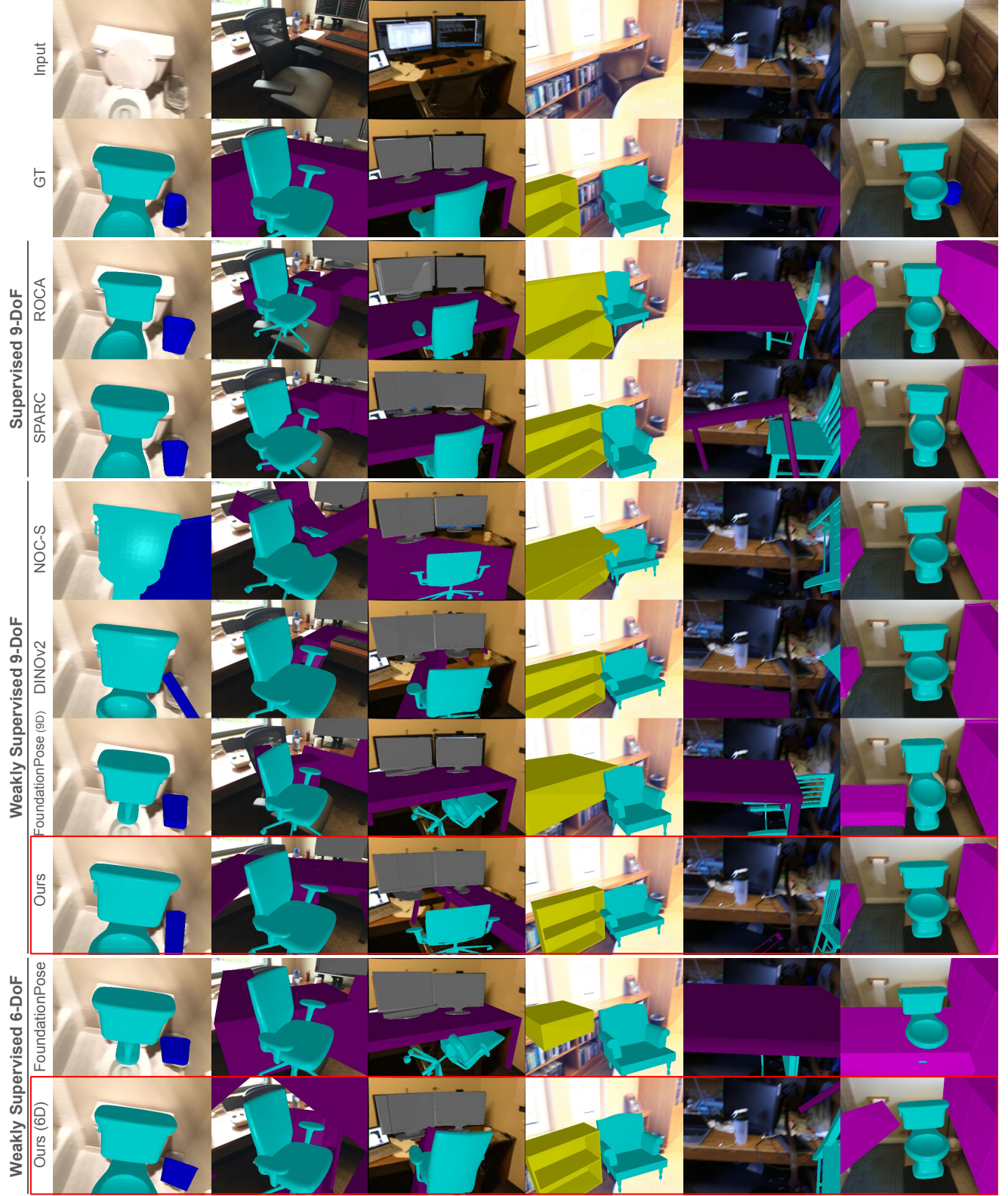
Figure 17. Random test samples from ScanNet25k. We compare entire-scene CAD alignment against 9-DoF supervised methods (SPARC [26] and ROCA [18]), 9-DoF weakly supervised methods (DiffCAD [16]), and 6-DoF weakly supervised baselines (FoundationPose [49])
