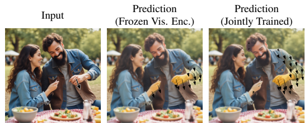
Figure B. Jointly training the vision encoder is important. We train a model with a frozen pretrained vision encoder. The model struggles with instance-specificity, predicting the same movement for the woman’s hand as it does for the man’s hand. When jointly training the vision encoder with the flow poke transformer, the man’s hand’s movement does not directly influence the woman’s hand.
