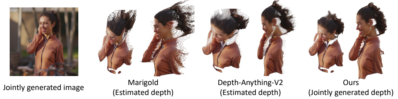
Figure S1. Comparison of 3D lifting results from our JointDiT, Marigold, and Depth-Anything-V2. The jointly generated depth from JointDiT leads to more coherent 3D shapes and better preservation of structural details compared to the estimated depths.
