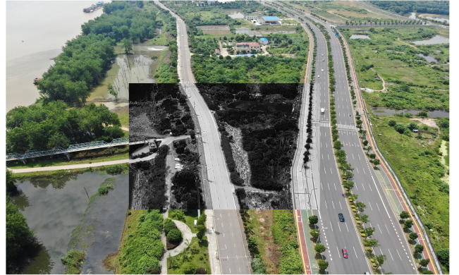
Figure 6. An example of misalignment in raw RGB-IR image pairs.
