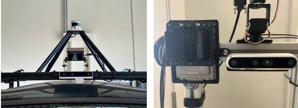
Figure 1. The two LiDAR-camera systems used for data collection. The left is for outdoor, and the right is for indoor.
