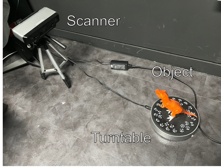
Figure S2. EinScan SP V2. An object is placed on turntable, and the scanner is looking at the object.
