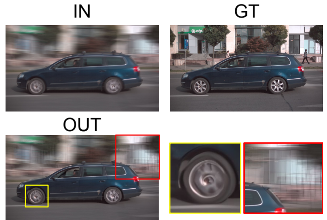
Figure 16. Qualitative analysis of FFTformer [14] on one frame of our MIORe dataset. Top-left quadrant displays the input blurry image. Top-right quarter shows the equivalent ground truth label. Bottom-left part represents the output of the model, and on the bottom-right side one may observe the highlighted degradations of the model. In this case, FFTformer creates a grid-like degradation due to the overwhelming blur intensity. It is to be noted that some particular movement types are underrepresented in multiple datasets that we compared to. In this particular case, we may notice how models trained on [20] are unable to correctly restore the spinning wheel . This effect is persistent with all the models we have benchmarked for motion deblurring.
