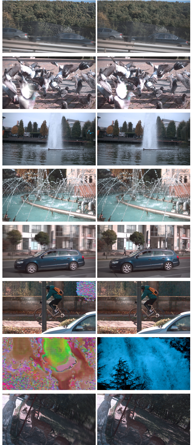
Figure 18. Qualitative analysis of NAFNet [4] on a sample frame of our MIORe dataset. Left column displays the output of the model, provided the blurry-rendered inputs, while on the right we have the corresponding ground truth sharp images.
