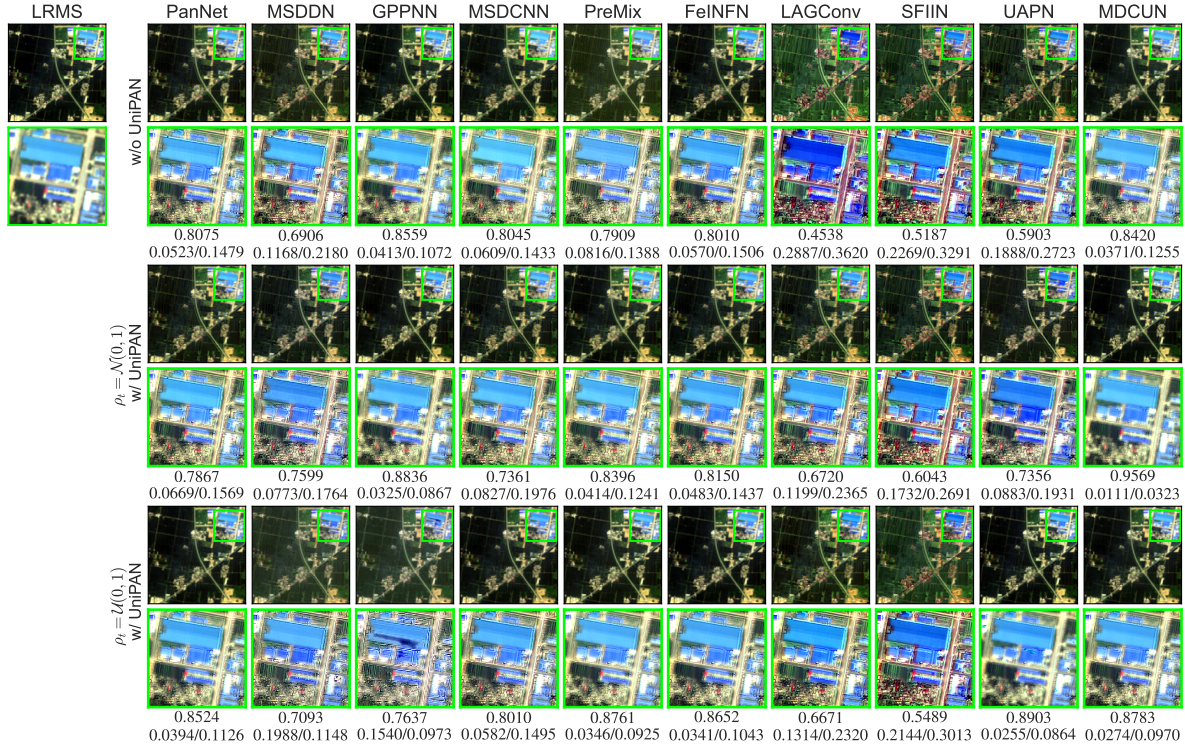
Figure 3. Generalization testing on GaoFen-1, the networks are trained on WorldView-3. The bright green box indicates the zoomed-in area. Below the zoomed-in image, the first line is the QNR value, and the second line is the D_\lambda/D_S value.
