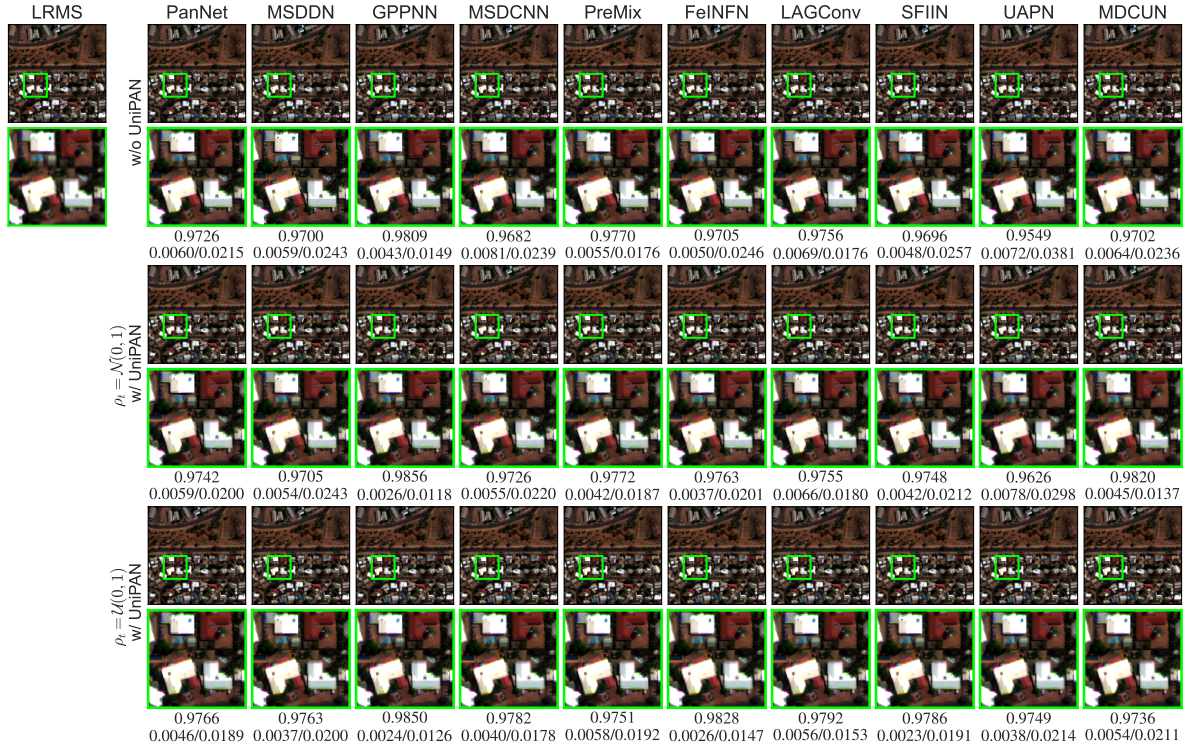
Figure 4. Full-resolution generalization testing on WorldView-4. The bright green box indicates the zoomed-in area. Below the zoomed-in image, the first line is the QNR value, and the second line is the D_\lambda/D_S value.
