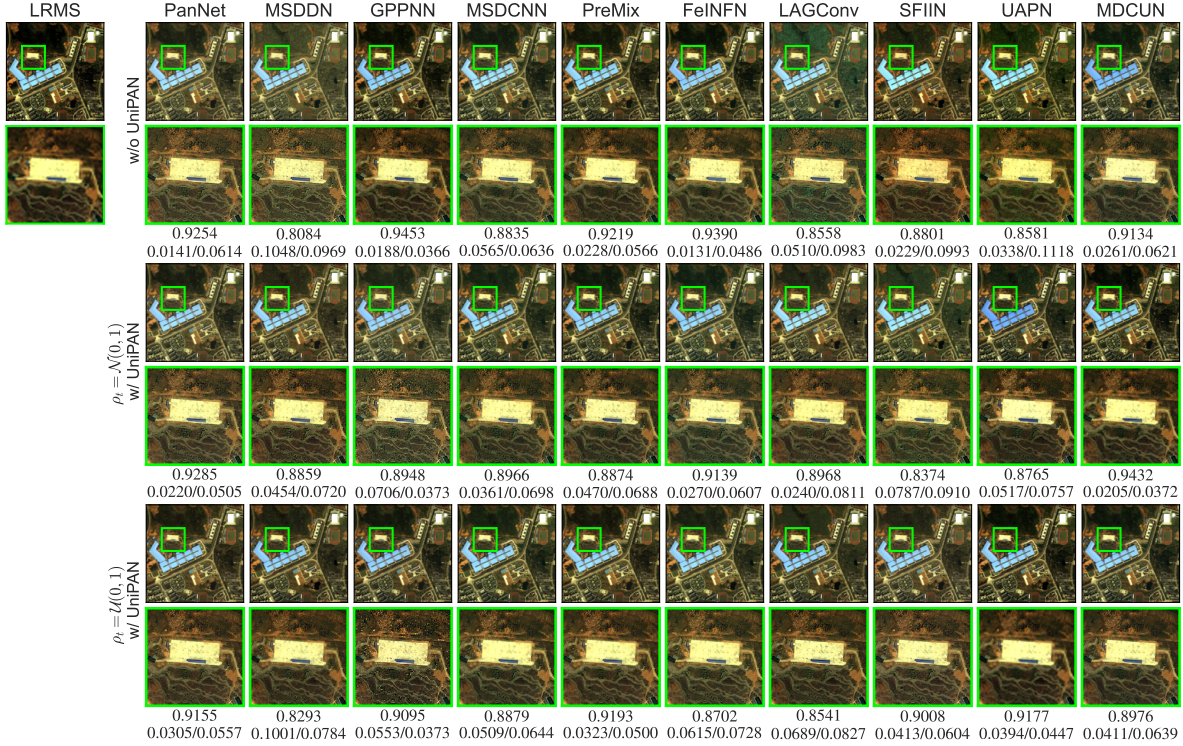
Figure 2. Generalization testing on IKONOS, the networks are trained on WorldView-2. The bright green box indicates the zoomed-in area. Below the zoomed-in image, the first line is the QNR value, and the second line is the D_\lambda/D_S value.
