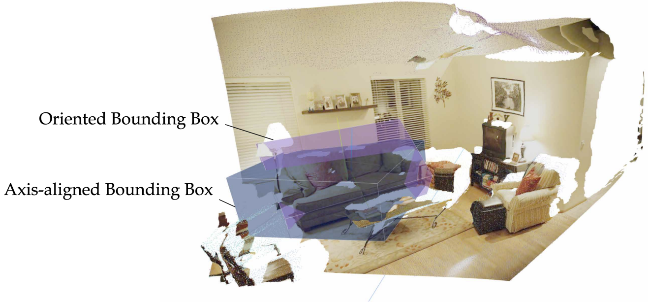
Figure 8. Comparative visualization of axis-aligned vs. oriented 3D bounding boxes, taken from the SpatialRGPT paper [27, Appendix K, Figure 11]. The object dimensions computed from AABBs can differ substantially from those computed from OBBs, depending on the object’s rotation. For sake of illustration, assume that the sofa is 2m wide and 0.8m deep. We then obtain the following altered object dimensions when using an AABB instead of an OBB, at different yaw rotation angles (i.e., considering 7-DOF bounding boxes that are gravity-aligned / parallel to the ground, as in CA-1M / CA-VQA): width \approx 2.1 m and depth \approx 1.7 m with 30^\circ rotation; width \approx 1.7 m and depth \approx 2.1 m with 60^\circ rotation; and width = 0.8m and depth = 2m with 90^\circ rotation (i.e., “full” rotation resulting in swapped dimensions).
