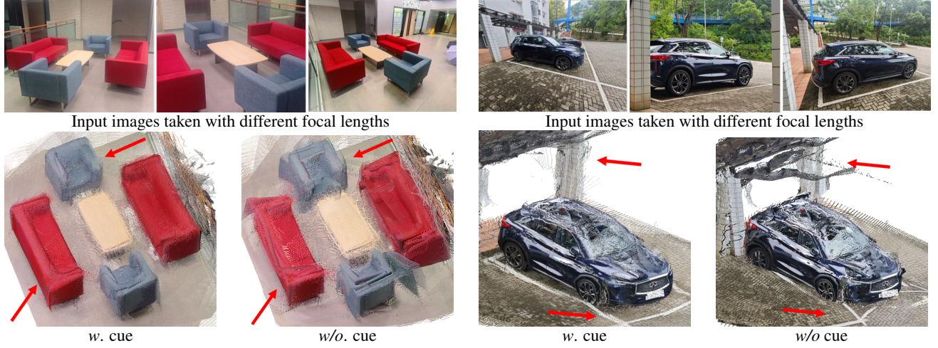
Figure 12. Sparse View 3D Reconstruction with Intrinsic Cues. We captured images with various focal lengths and present the reconstruction results. With intrinsic cues, our method achieves more accurate and better-aligned reconstructions.
