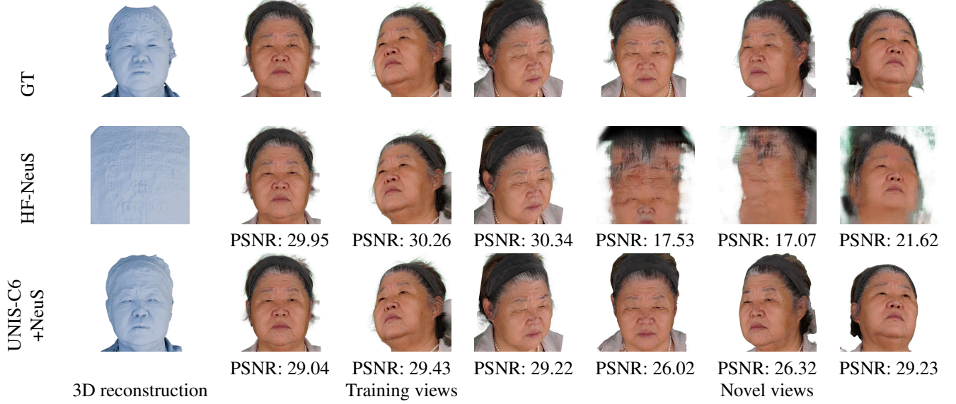
Figure 7. Sparse-view reconstruction of a human head. The input consists of five images with views covering the human face. We adopt a two-stage training strategy, using NeuS in the first stage followed by UNIS-C6 in the second stage, to effectively learn both geometry and appearance. This figure presents the reconstructed geometry alongside six rendered images: three from training views and three from novel views, with PSNR values reported to quantify rendering quality for each method. Due to the limited number of views, HF-NeuS tends to overfit to colors in the training views, producing high-quality renderings for these views. However, its inability to accurately reconstruct geometry leads to a significant drop in performance for novel views. In contrast, our method, while slightly underperforming in PSNR for training views, effectively reconstructs both geometry and appearance, achieving much better results on novel views.
