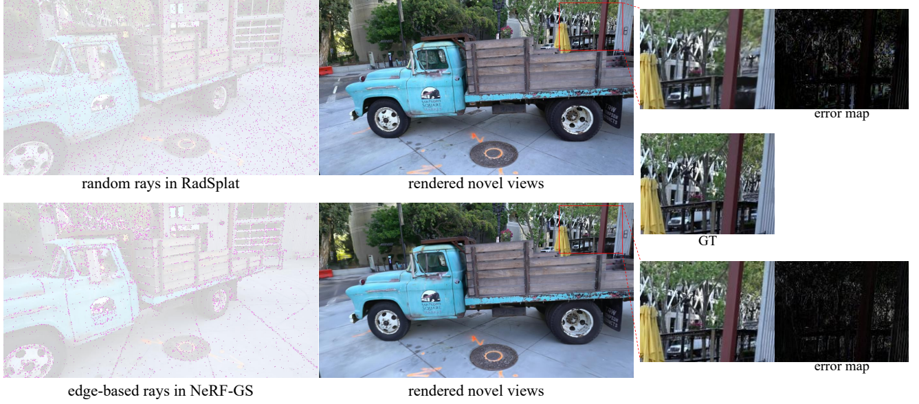
Figure 2. Comparison of initialization with RadSplat. NeRF-GS focuses more on the contours of the scene during ray sampling, alleviating the burden of position optimization in the GS branch while achieving superior visual results in regions with complex textures.
