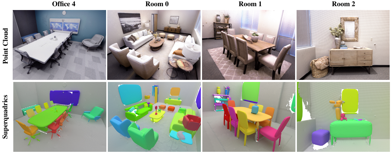
Figure 13. Qualitative Results on Replica [45]. We show results on different scenes from Replica. In the first row we show a rendering of the input mesh, while on the second row we show the output superquadrics. We visualize different object instances with different colors.
