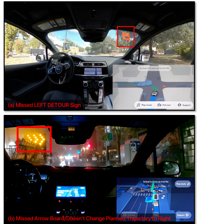
Figure 1. Examples of work zone failures in a commercial self-driving vehicle. While obtaining detailed failure reports of self-driving cars is infeasible, customers of these companies regularly post failure cases on social media. (a) The car failed to recognize and observe a sign that mentions “DETOUR” and has a left arrow graphic (Link). (b) The car fails to recognize and observe the Arrow Board, then fails to analyze the situation and finally does not change the predicted pathway in response (Link).
