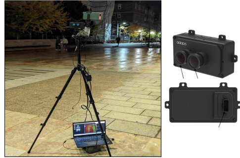
Figure 2. Outdoor Camera Setup: The Figure shows the front view of our Adaps camera setup (left) and the sensor (right).
