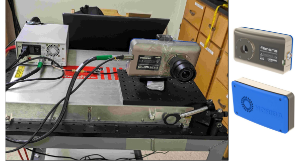
Figure 1. Indoor Camera Setup: The Figure shows the front view of our FLIMera camera setup (left) and the sensor (right).
