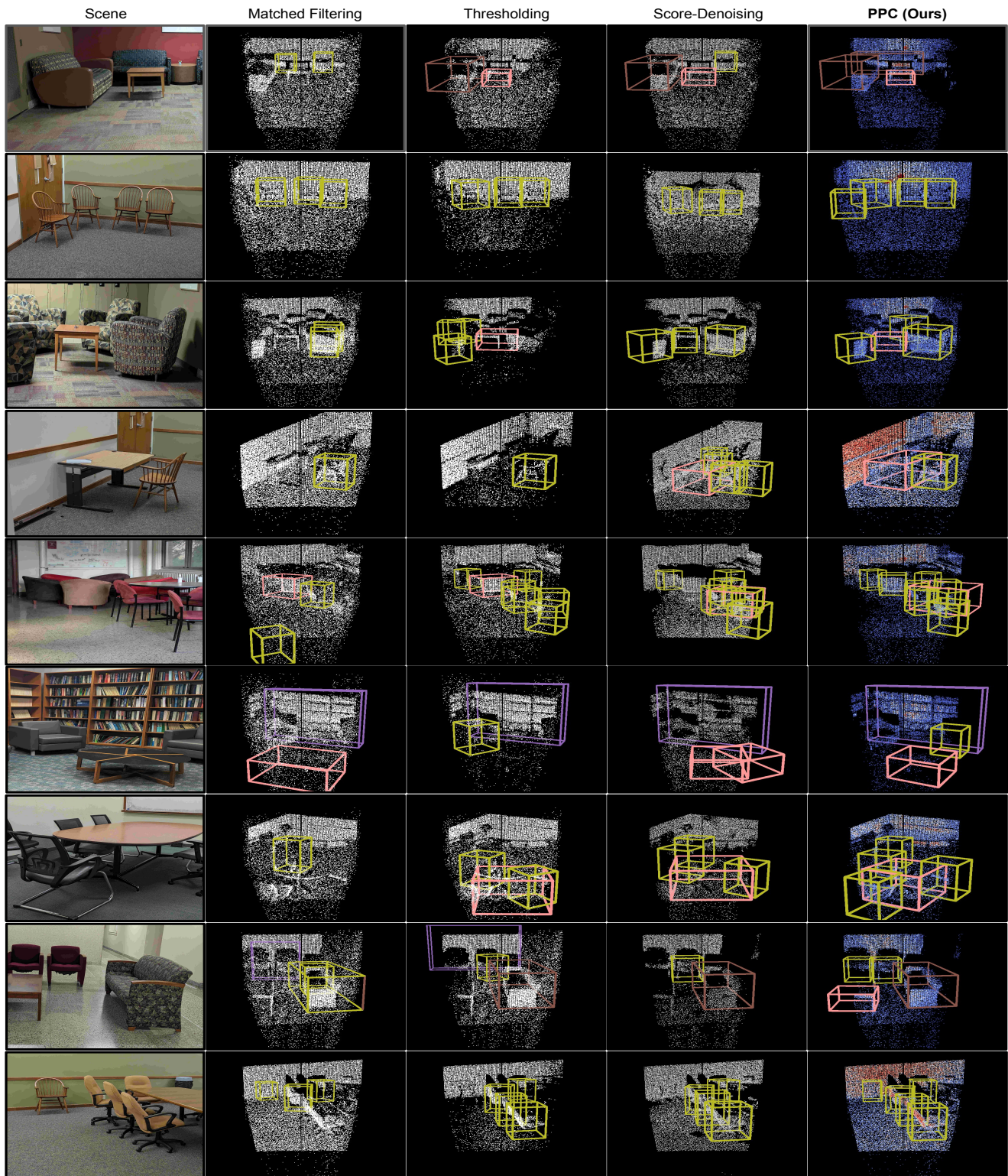
Figure 4. 3D Detection Results on Real Indoor Captures: Figure compares our method with the baselines under challenging low SBR conditions. Baselines fail to detect many small and farther objects, e.g. chairs in the back, in many scenes. PPC detects most objects ( e.g. chair, table, and couch) with tight bounding boxes.
