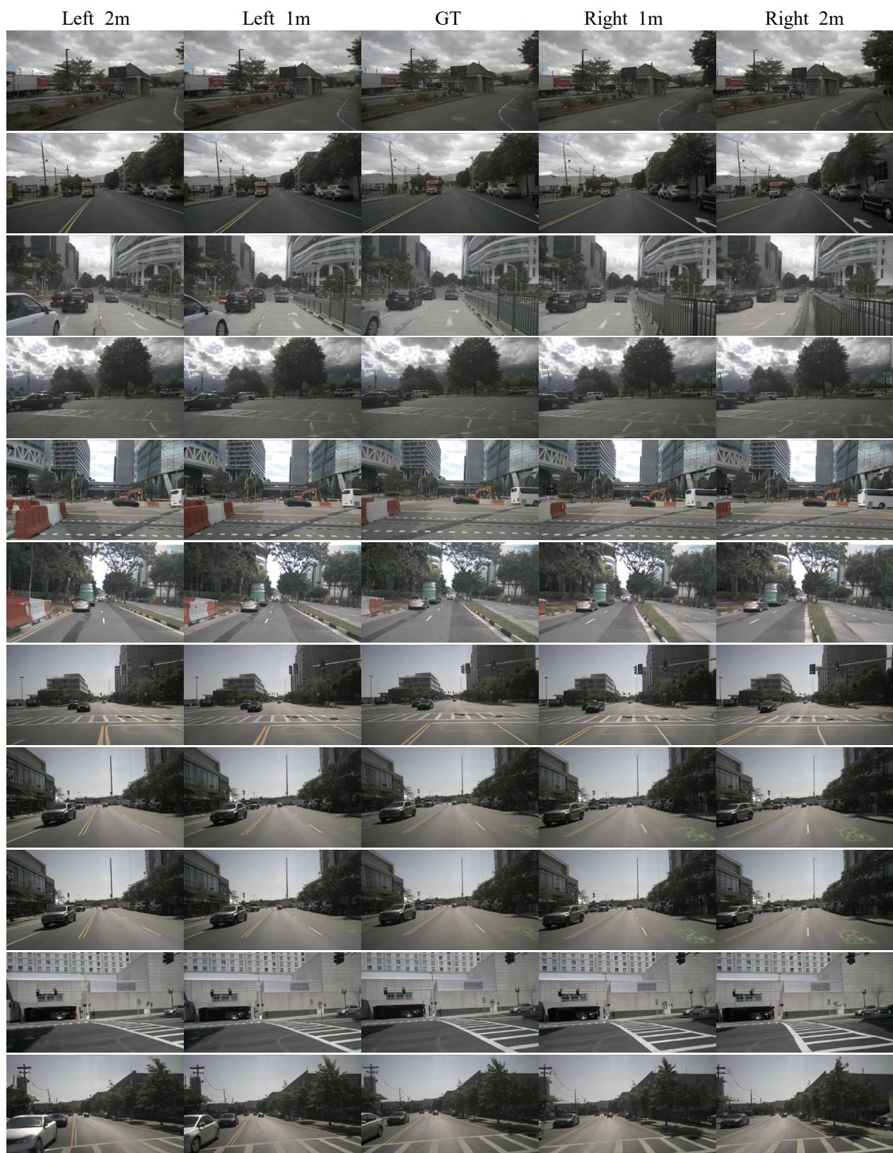
Figure 13. Additional visualizations of spatial novel view synthesis using DiST-S. We present NVS results of DiST-S from various shifted viewpoints, demonstrating our method’s ability to generate photorealistic images with high consistency to the original scene.
