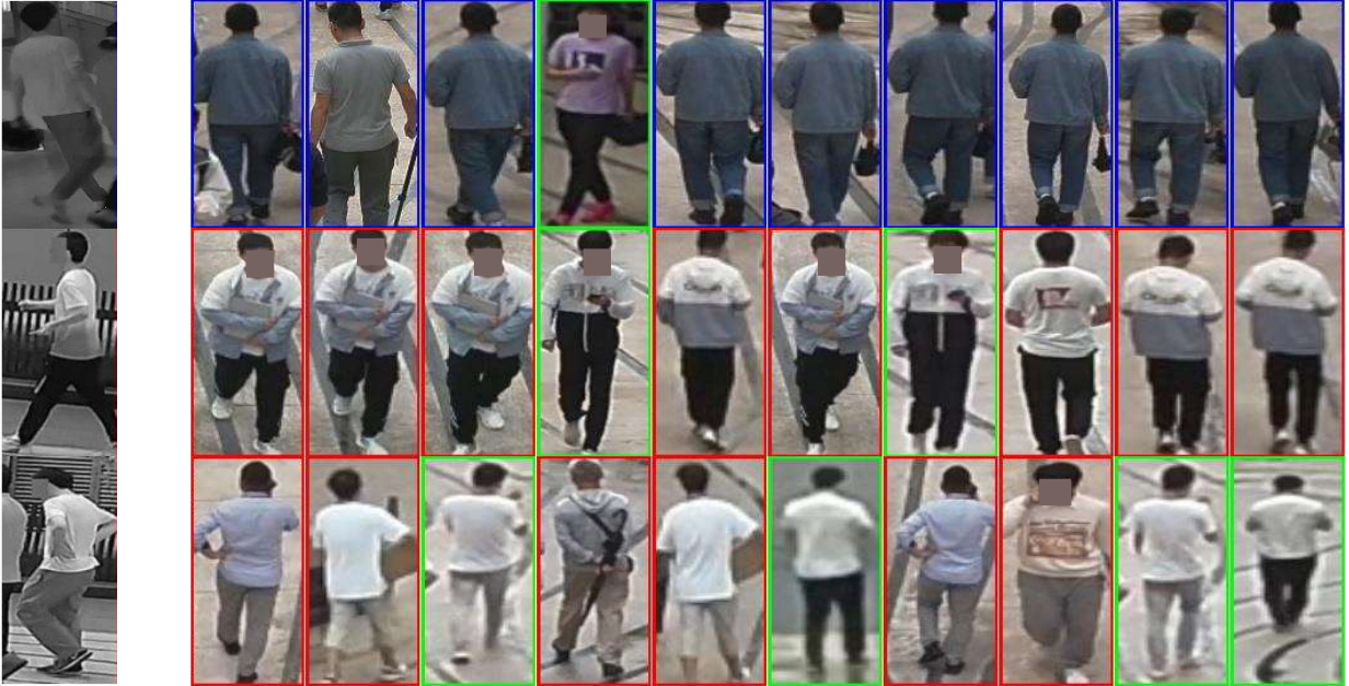
Figure 7. Visualization of OTLA-ReID retrieval results. Query images are from ground infrared cameras and gallery images are from UAV RGB cameras. Green, red and blue rectangles indicate correct, wrong retrieval results and distractors, respectively.
