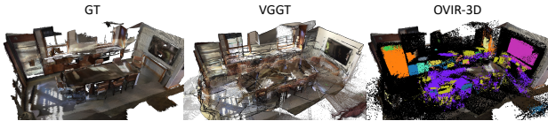
Figure 5. 3R baseline qualitative result. Comparison between (left) ground-truth ScanNet scene, (middle) VGGT 3D reconstruction using only RGB images and poses, and (right) OVIR-3D segmentation result on the VGGT output. The reconstruction lacks fine-grained indoor geometry, resulting in inaccurate 2D-3D matching and degraded segmentation quality.
