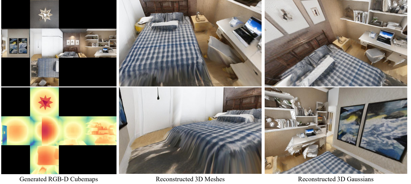
Figure 4. Panorama-to-3D scene reconstruction. Based on the RGB-D cubemap generated by DreamCube, we can reconstruct the corresponding 3D scenes in seconds and obtain both 3D mesh and 3D Gaussian [3] representations.
