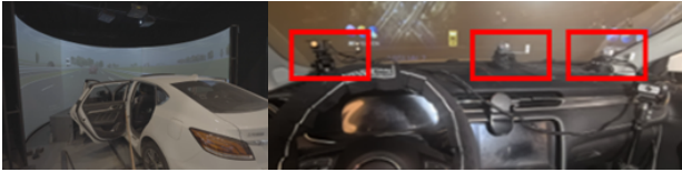
Figure S-1. Experimental Equipment: High-fidelity driving simulator (left) and in-vehicle eye-tracking system (right)
