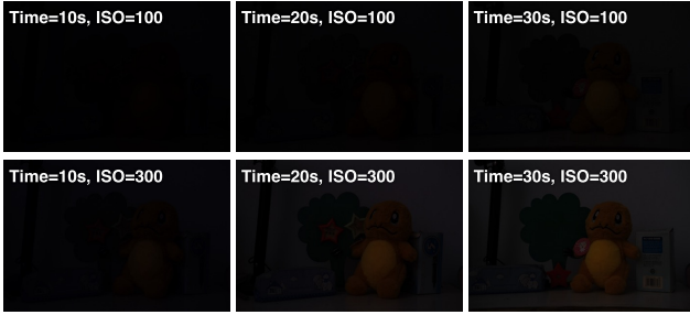
Figure S5. Capturing images in the realistic extremely dark scene using various camera parameters. These images are in sRGB format produced by camera default ISP in a 0.001lux-0.01lux scene.
