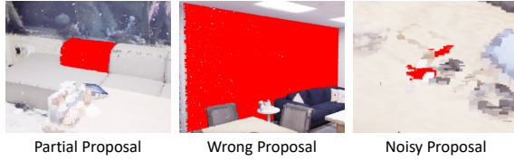
Figure 2. Visualization of filtered proposals by using the Standardized Maximum Similarity (SMS) score. The SMS score effectively filters out partial proposals (e.g., only part of a sofa is covered), incorrect proposals that do not match any text queries (e.g., "wall" class not included in the evaluation set), and noisy proposals lacking meaningful object representation.
