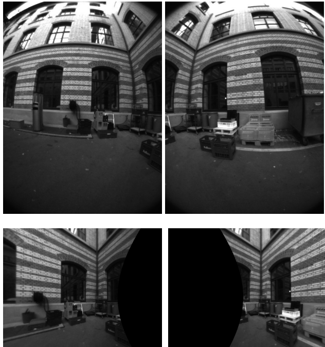
Figure 1. The overlap of the two SLAM cameras is severely limited, making it hard to evaluate in horizontal stereo mode. Top: The original SLAM image pair, Bottom: The SLAM image pair after stereo rectification.
