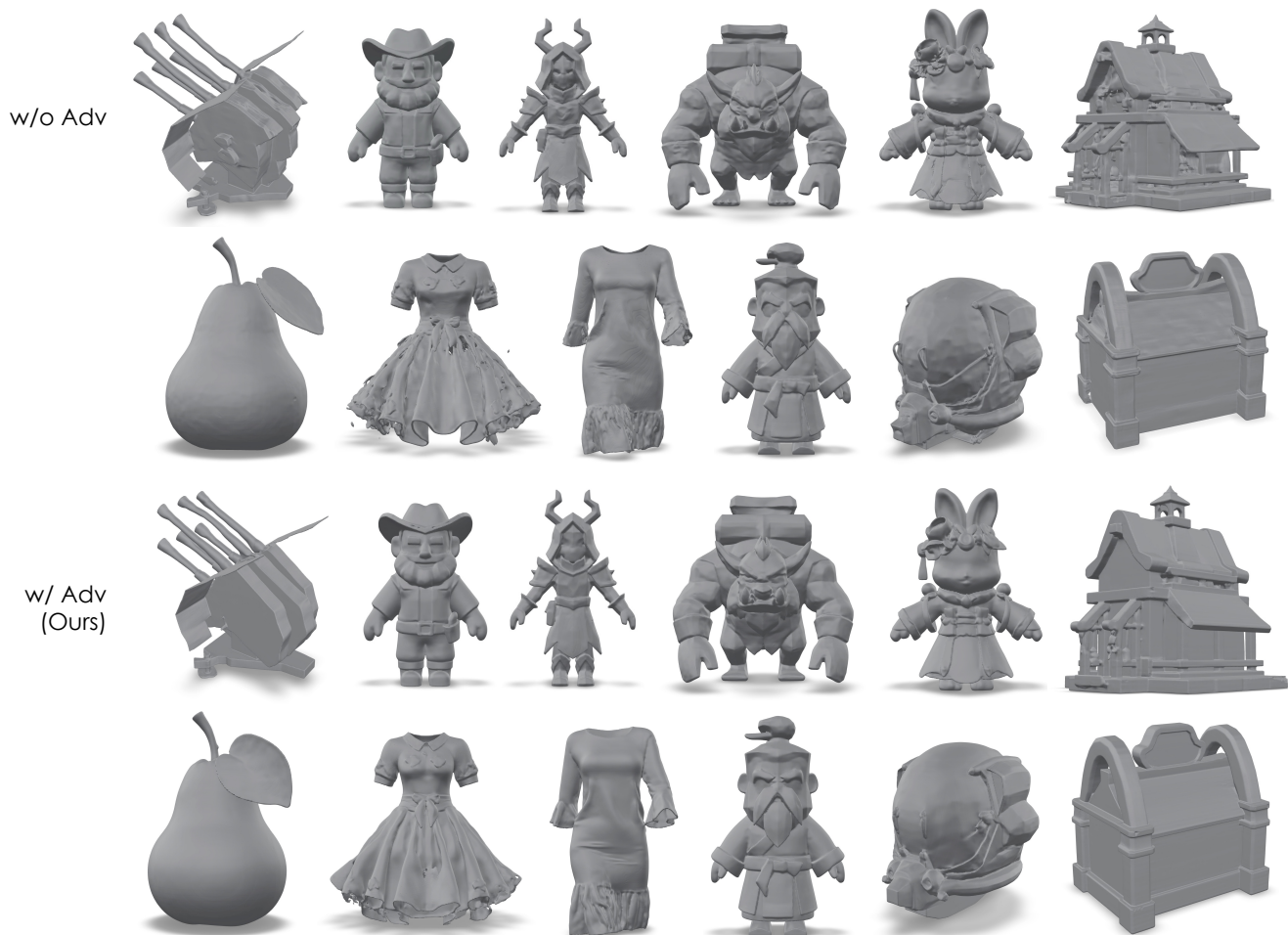
Figure 10. Visual comparison of models with and without adversarial finetuning . All other distillation stages are used. It demonstrates that the predicted meshes are more accurate and smooth after adversarial finetuning.
