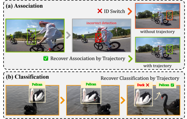
Figure 1. Trajectory information can enhance both association and classification by helping to recover associations disrupted by inaccurate or missed detections (as shown in (a)) and by correcting incorrect classifications (as shown in (b)).
