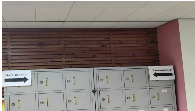
Figure 4. Examples of placing reference objects in the data alignment pipeline. To mitigate misalignment between each GT-LQ frames, we place recognizable reference objects as start-marker and end-marker before and after the uniform moving phase.
